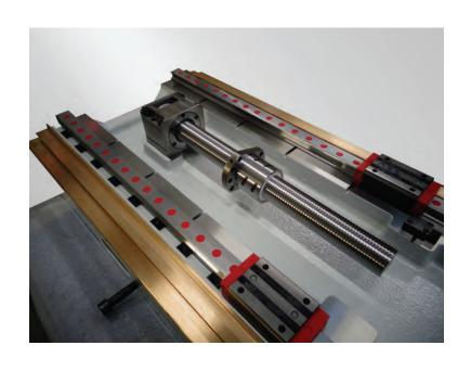
Both the transverse (X) axis and the longitudinal (Z) axis can be equipped with a brushless motor coupled to a ball screw or with linear motors controlled by an absolute optical scale. Support groups are in place for use of the customer's preferred system.
