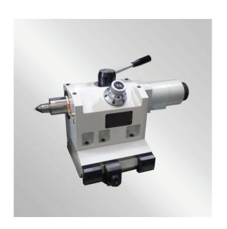
The tailstock unit has everything you need: controlled movement manually by lever or automatically by pedal; pushing on the piece adjustable by spring or hydraulic. The cylindricity adjustment of the pieces is done with a practical front knob equipped with an optical scale.
